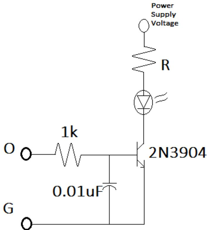
The value of R depends on the maximum anticipated power supply voltage (including failure modes) to protect the LED and the 2N3904 against over current.
