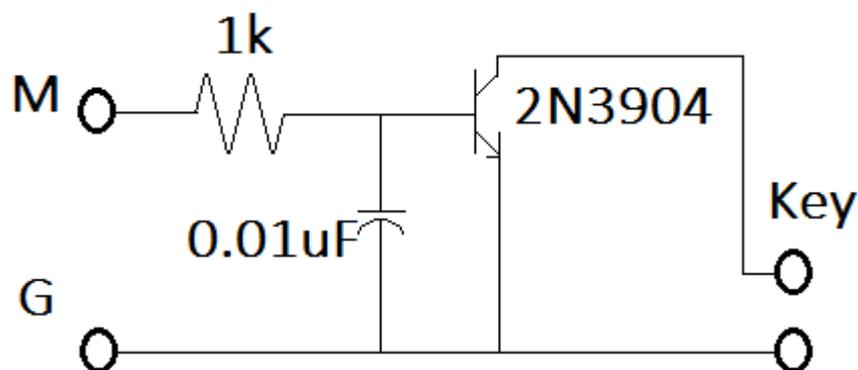
A code oscillator can be generally keyed by a simple straight key. A straight key is a simple switch that shorts two contacts. Here we are using the 2N3904 as an inverter and to provide enough key current to drive many code oscillators. Optical isolation might also be used but output current from the optical isolator may not be enough to directly drive the oscillator.
