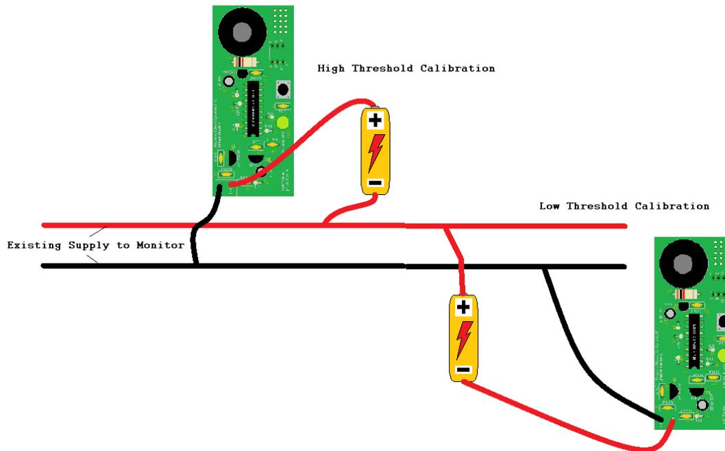
Looking at the diagram we can see how to use a single 1.5 volt battery to add and subtract 1.5 volts from an existing supply. Calibration of the high and low thresholds in this way gives a small margin around the voltage at the time of calibration.
