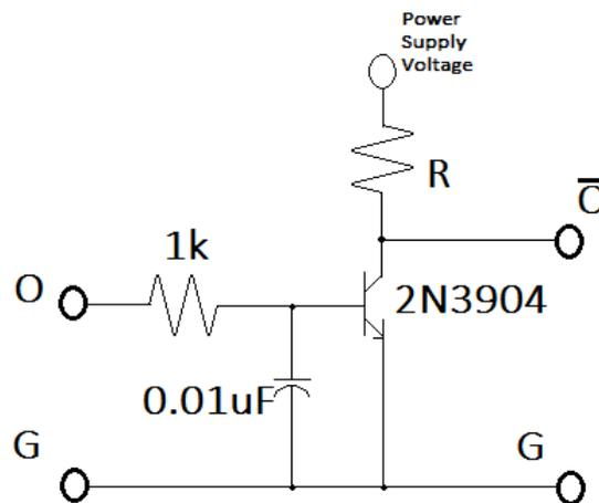
Any of the signals can be inverted simply with the circuit above. In this case the output logic level will be the inverse of *O*. This may be useful if a true logic signal is needed to indicate that the voltage is OK. Resistance and power values for *R* should be determined for driving downstream logic requirements. If we want to drive an LED, however, *R* can be determined as shown here.
