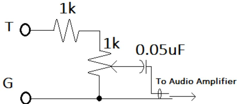
The above circuitry somewhat isolates the audio output from the microcontroller. It also provides a bit of adjustable attenuation for the audio. Be aware that AC hum may be present here in the form of ground loop hum. An isolation transformer can help. In addition amplification locally to VT can cut down on ground loop induced hum.
