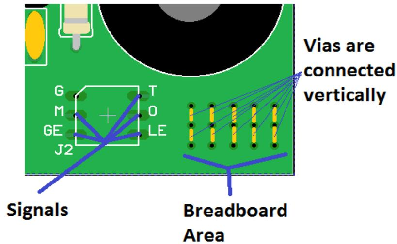
The Volt Tattler V1.01 has the signals next to a small breadboard area. It is hoped that this small area will assist in getting signals from the board for use by equipment downstream. The breadboard area is a set of vias vertically connected. Parts may be inserted here for experimentation and implementation purposes.
