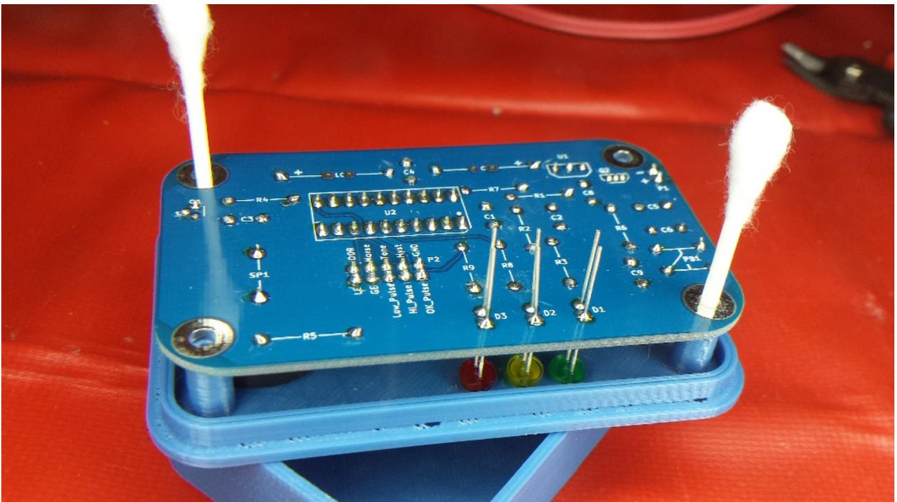
Then simply remove the centering tools (swabs in this case). There are no screws holding the board into the case. It is held by posts printed into the lid and base. The lid simply snaps on.
