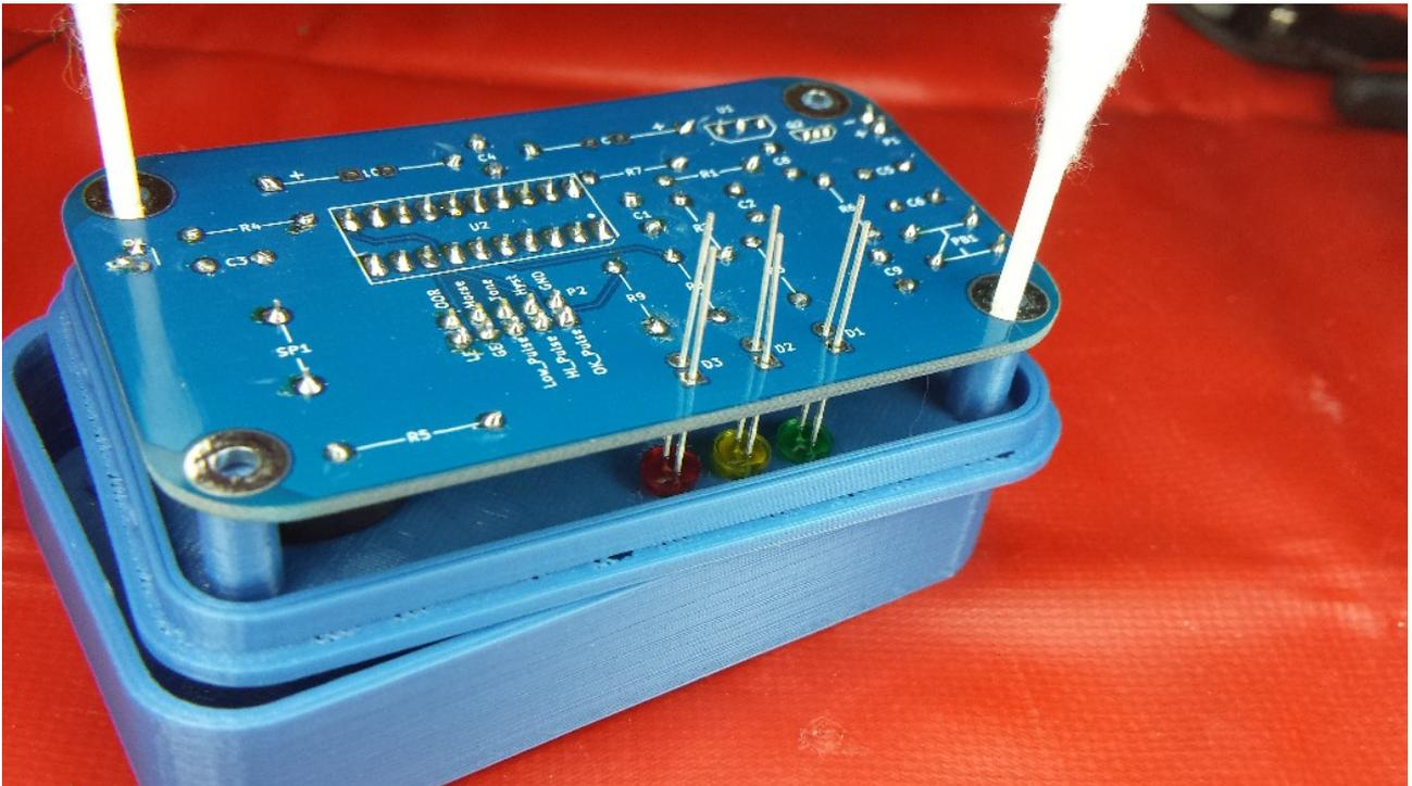
Next solder in the LEDs. Solder all 6 leads.
