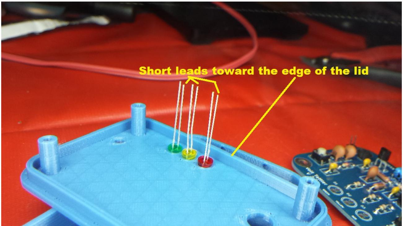
Tip the lid upside down and insert the LEDs in the holes as shown. Do not mix up the colors, red going near the center of the lid. Put the leads so that the short lead (and the flat side of the diode) is toward the side of the lid as shown.
