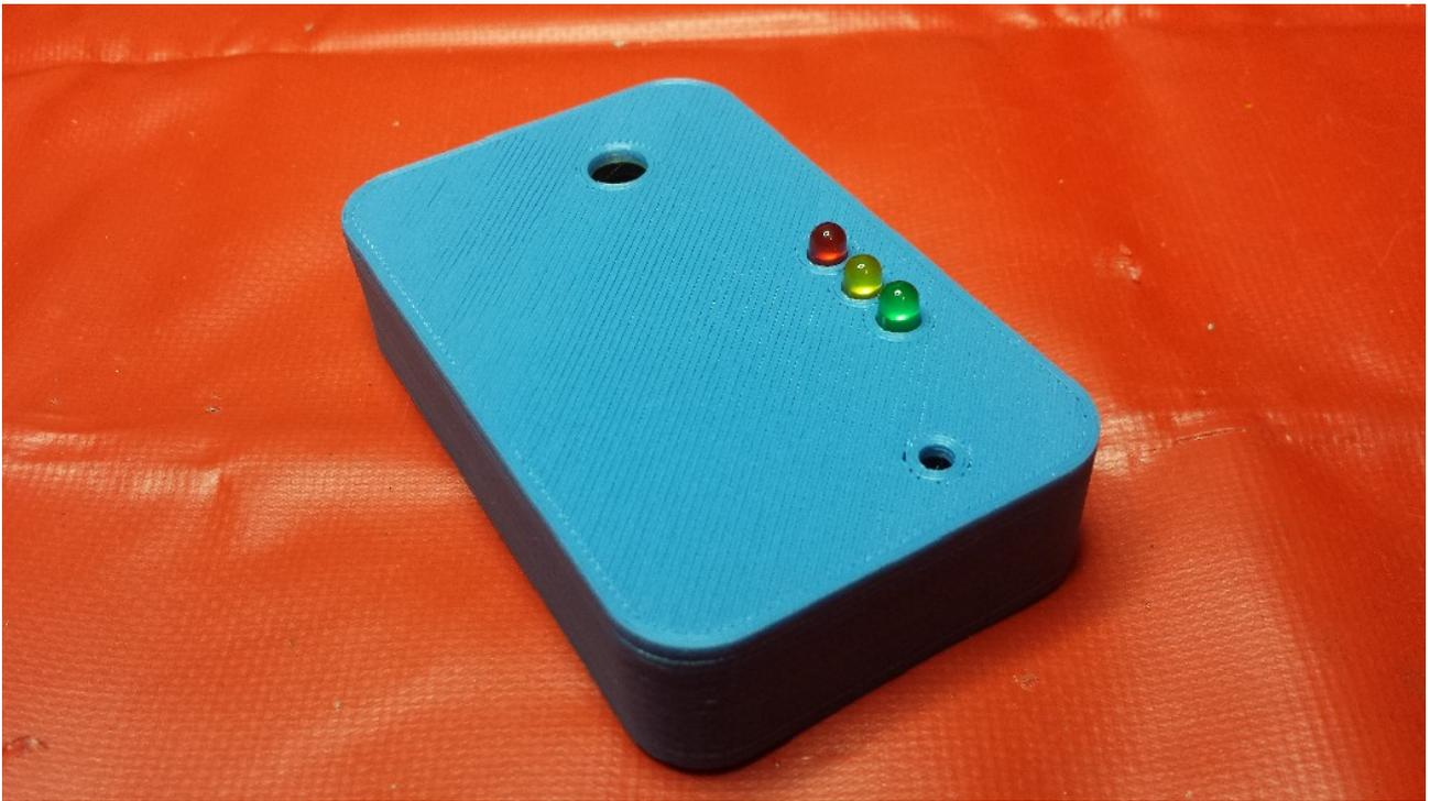
I have not added holes for the power leads, leaving them to be drilled by the user. We each may have our own requirements for connecting to the VT2. A little hot glue as a strain relief for the wires coming into the case may be a good idea.
