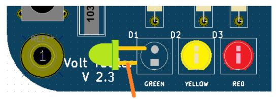
Note the short lead and the flat side of the LED must go toward the edge of the board.
