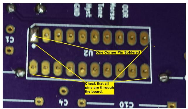
If all of the pins are viewed as through the board as in the above image carefully solder the remaining pins avoiding solder bridges between the pins and adjacent traces.
