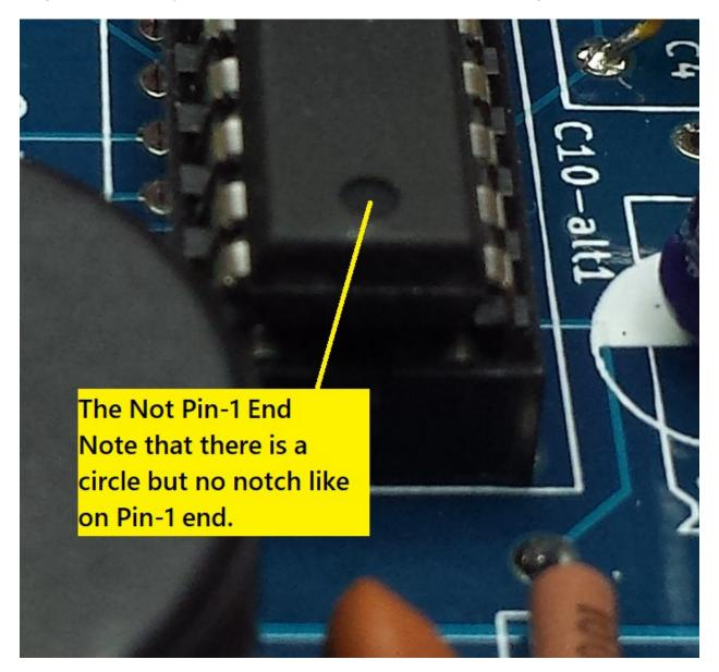
Carefully aligning the pins can prevent bending a pin off to the side or underneath the chip.
