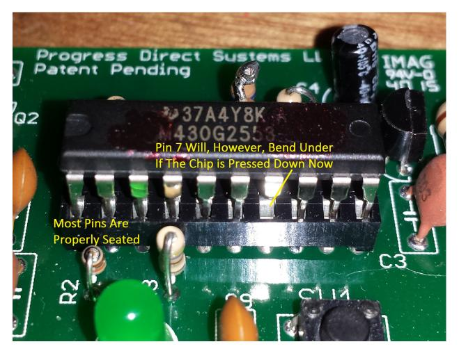
In the above picture the builder is headed for trouble. Pin 7 of the chip is not pointing down into the socket but tucked a bit back under the chip. When this builder pushes down on the chip to seat it into the socket, pin-7 will fold under the chip and not connect. This may cause issues even though the chip seemed to seat solidly. Check each pin for proper position before attempting to seat the chip into the socket.
