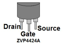
In normal operation Q1 is turned on so there should be little voltage difference between the Drain and Source. If Q1 is not turned on check its orientation along with R6 and C5 for solder bridges and bad solder joints.
