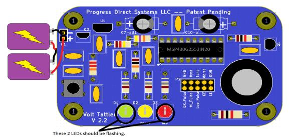
In this connection, at power up, a new Volt Tattler 2 should announce the Morse 'R'(.-.) then repeat Morse 'H' (....). The Green and Red LEDs should also be flashing.
